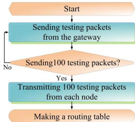
Figure 4 The flowchart of the establishment of the routing table.
