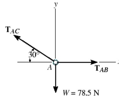
$$\Sigma F_x = 0: T_{AB} - T_{AC} \cos 30^\circ = 0$$
