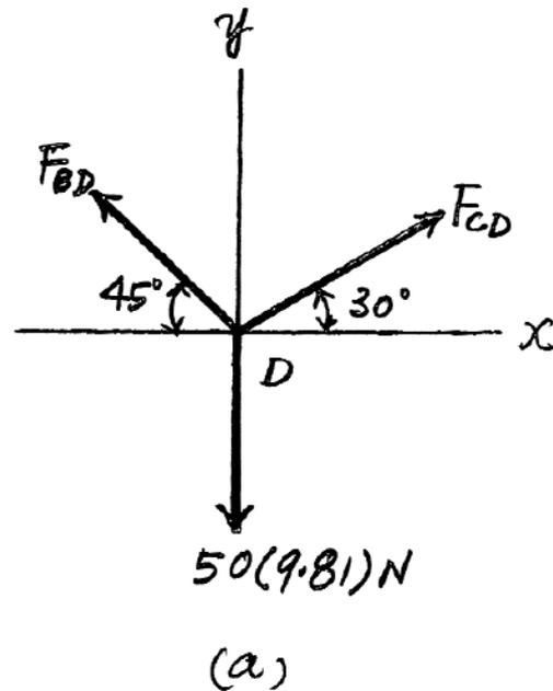
**Equations of Equilibrium:** First, we will apply the equations of equilibrium along the  $x$  and  $y$  axes to the free-body diagram of joint  $D$  shown in Fig. (a).
