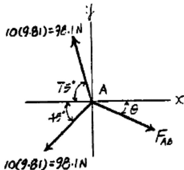
**Free Body Diagram :** The tension in the cord is the same throughout the cord, that is  $10(9.81) = 98.1 \text{ N}$ .
