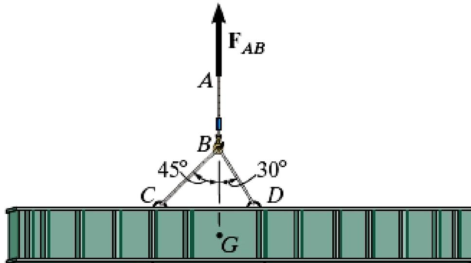
**Equations of Equilibrium:** The girder is suspended from cable  $AB$ . In order to meet the conditions of equilibrium the tensile force developed in cable  $AB$  must be equal to the weight of the girder. Thus,
