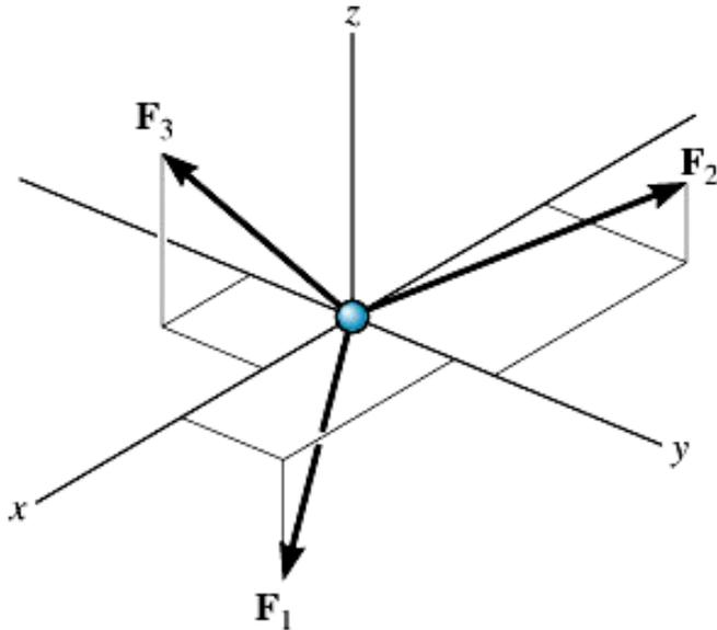
$$\underline{\Sigma F} = \Sigma F_x \underline{i} + \Sigma F_y \underline{j} + \Sigma F_z \underline{k} = 0$$
